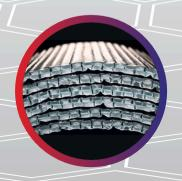
NAAD® AD80 NAAD AD80 comes with a double layer of 4mm thick Bubble sheet laminated
