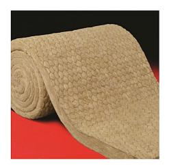
**SUNR**©CK Lightly Resin Bonded (LRB) Stonewool mattresses are made out of molten rocks (Basalt) transformed into fibres and then bonded with thermosetting binder forming mattress and then it is stitched with one side or both sides GI or SS hexagonal wire netting.
